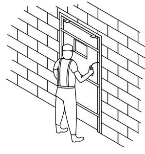
MASK WALL NEXT TO FRAME ALL AROUND AND INJECT SMALL AMOUNT (ONE SECOND SHOT) BETWEEN FRAME & WALL AT EACH HINGE, STRIKE, & TOP AND BOTTOM OF FRAME. DO NOT OVER FILL.
