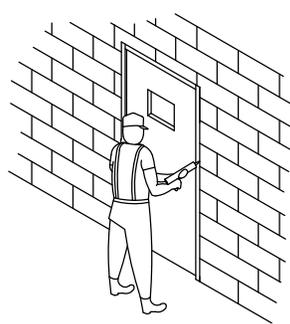
INSTALL FASTENERS AS REQUIRED. CAULK JOINT BETWEEN FRAME & WALL WITH SPECIFIED SEALER.
