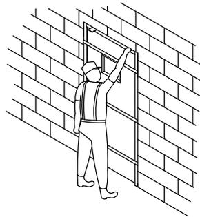
MAINTAIN UNIFORM CLEARANCE AROUND DOOR & FRAME. SLIDE WOOD SHIMS BETWEEN JAMB AND WALL AT TOP UNTIL ASSY IS SNUG.
