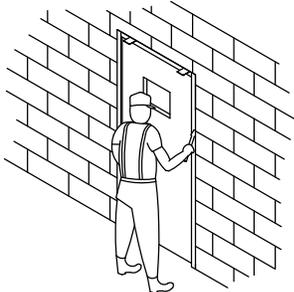
AFTER 4-6 HRS. REMOVE STRAPS & PULL DOOR OPEN. TRIM FOAM & REMOVE TAPE. RAKE FOAM BACK 1/8" & TRIM AWAY EXCESS SHIMS & STRAPS WITH A WOOD CHISEL OR A KNIFE.
