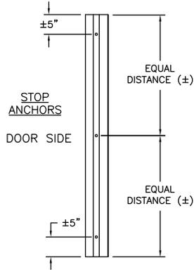
**Optional Stop anchors**- Same as above except field drill 3/8" hole in jamb stop and structure. Place 3/8" anchor 5" or 6" from each end of frame to start and then 3' o.c. Specify on order.
