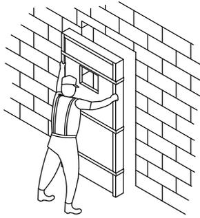
SLIDE ASSEMBLED DOOR & FRAME INTO EXISTING OPENING. CHECK HANDING PER PLANS.
