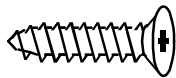
#12 x 1-1/4" (min) SHEET METAL SCREW INTO JAMB (FURNISHED BY CHEM-PRUF FOR BUTT HINGES, FURNISHED BY HINGE MANUFACTURER FOR CONTINUOUS HINGE)
