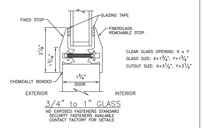
NOTE: CHEM-PRU PULTRUSION STANDARD WINDOW KIT SIZES ARE 12x12, 8x30, 24x24, 24x30.
